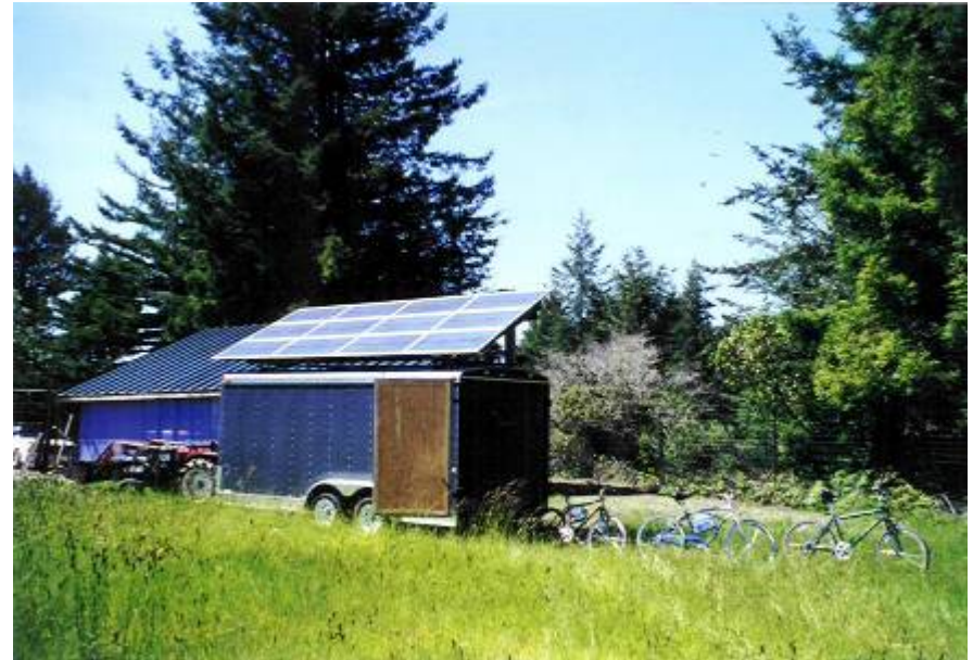
16 bike solar powered charging trailer
