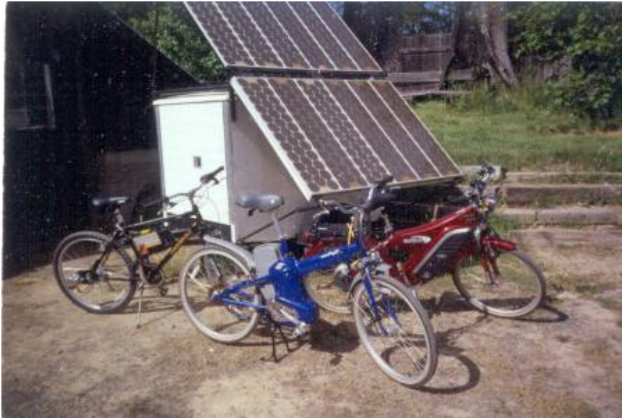
Solar powered charging electric bikes
